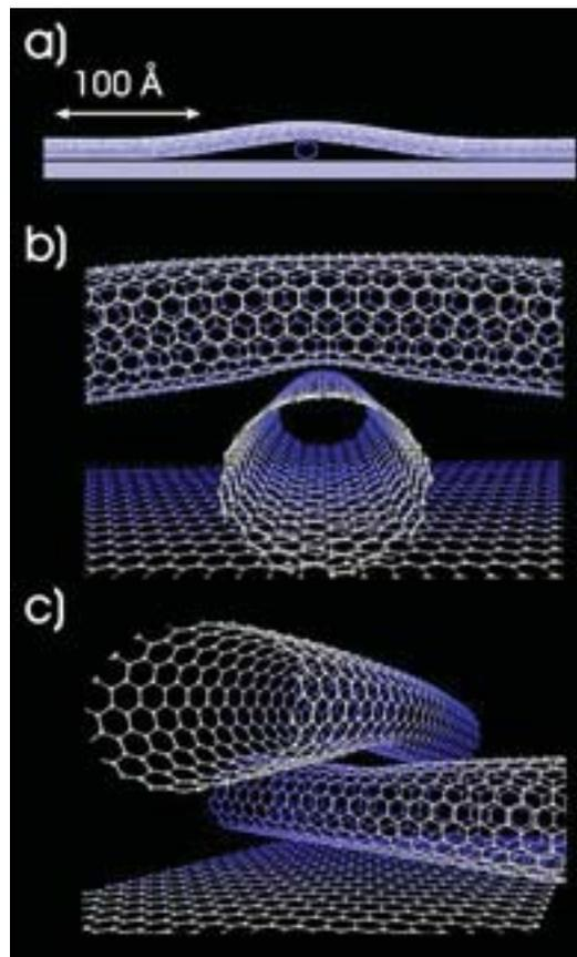
Nanotubes are tiny tubes about 10,000 times thinner than a human hair. They consist of rolled up sheets of carbon hexagons. Discovered in 1991 by researchers at NEC, they have the potential uses as minuscule wires or in ultrasmall electronic devices and are very powerful conductors of electrical current.
