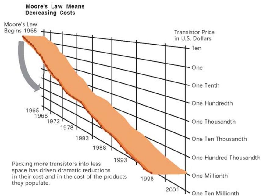
tinue into the future. Chip manufacturers continue to miniaturize components. Intel has recently changed its manufacturing process from 0.13-micron component size (a micron is a millionth of a meter), introduced in 2002, to a newer 90-nanometer process in 2004 (a nanometer is a billionth of a meter). With a size of about 50 nanometers, today's transistors should no longer be compared to the size of a human hair but rather to the size of a virus, the smallest form of organic life.
